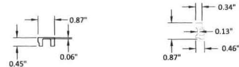
1 LOCK RAIL TOP ALUMINUM 2 LOCK MEETING RAIL ALUMINUM 3 BOTTOM LIFT RAIL & SASH ALUMINUM
